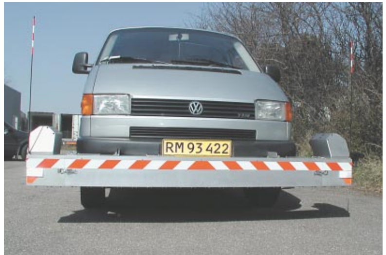
THE DYNATEST ROAD SURFACE PROFILER (RSP) IS CAPABLE OF REAL TIME CONTINUOUS HIGHWAY-SPEED MEASUREMENTS OF LONGITUDINAL PROFILE
