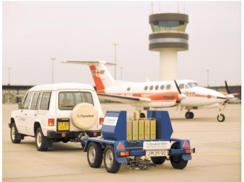
PAVEMENT DEFLECTION MEASUREMENTS USING THE DYNATEST FWD AND HWD FOR HIGHWAYS AND AIRFIELDS
